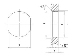
Installation direction: o-ring sits on chamfer.
